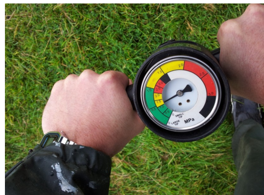
Taking penetrometer readings at Fferm y Glyn
